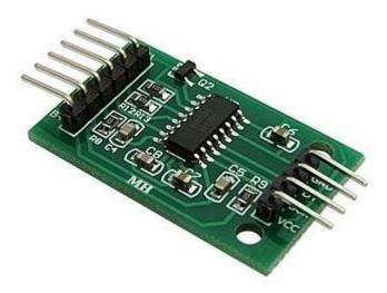
This module adopts hx711 4-bit high precision A/D converter chip, a chip specially designed for high precision electronic scale. It has two analog input channel. Internal is integrated with 128 times programmable gain amplifier. Input circuit can be configured to bridge type (such as pressure, weighing) sensor mode. It is an ideal, high precision, low cost, front-end sampling module;
